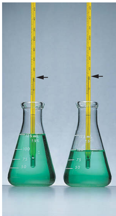
FIGURE A.2 Mass is an extensive property, but temperature is intensive. These two samples of iron(II) sulfate solution were taken from the same well-mixed supply; they have different masses but the same temperature. (W.H. Freeman photo by Ken Karp.)
