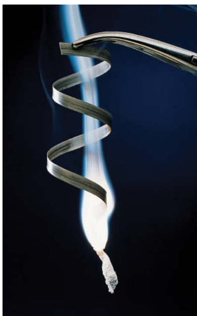
FIGURE 3 When magnesium burns in air, it gives off a lot of heat and light. The gray-white powdery product looks like smoke. (©1991 Richard Megna—Fundamental Photographs.)
