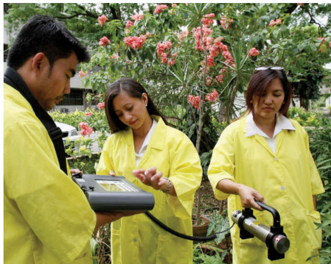
FIGURE 7 Scientific research today often requires sophisticated equipment and computers. These scientists are using a portable gamma spectrometer to measure gamma radiation levels near Quezon City in the Philippines. (Bullit Marquez/AP Photo.)
